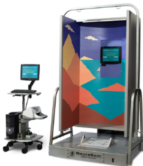
Figure 4. The Balance Master system used for assessing balance and motor function in participants before and after the intervention. This system measures postural stability, dynamic balance, and functional performance and was used as part of the outcome measures for both the soft robotic exoskeleton and conventional rehabilitation groups throughout the study.
