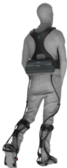
Figure 1. Yrobot Relink soft robotic exoskeleton used for soft robotic exoskeleton–assisted overground walking training.
