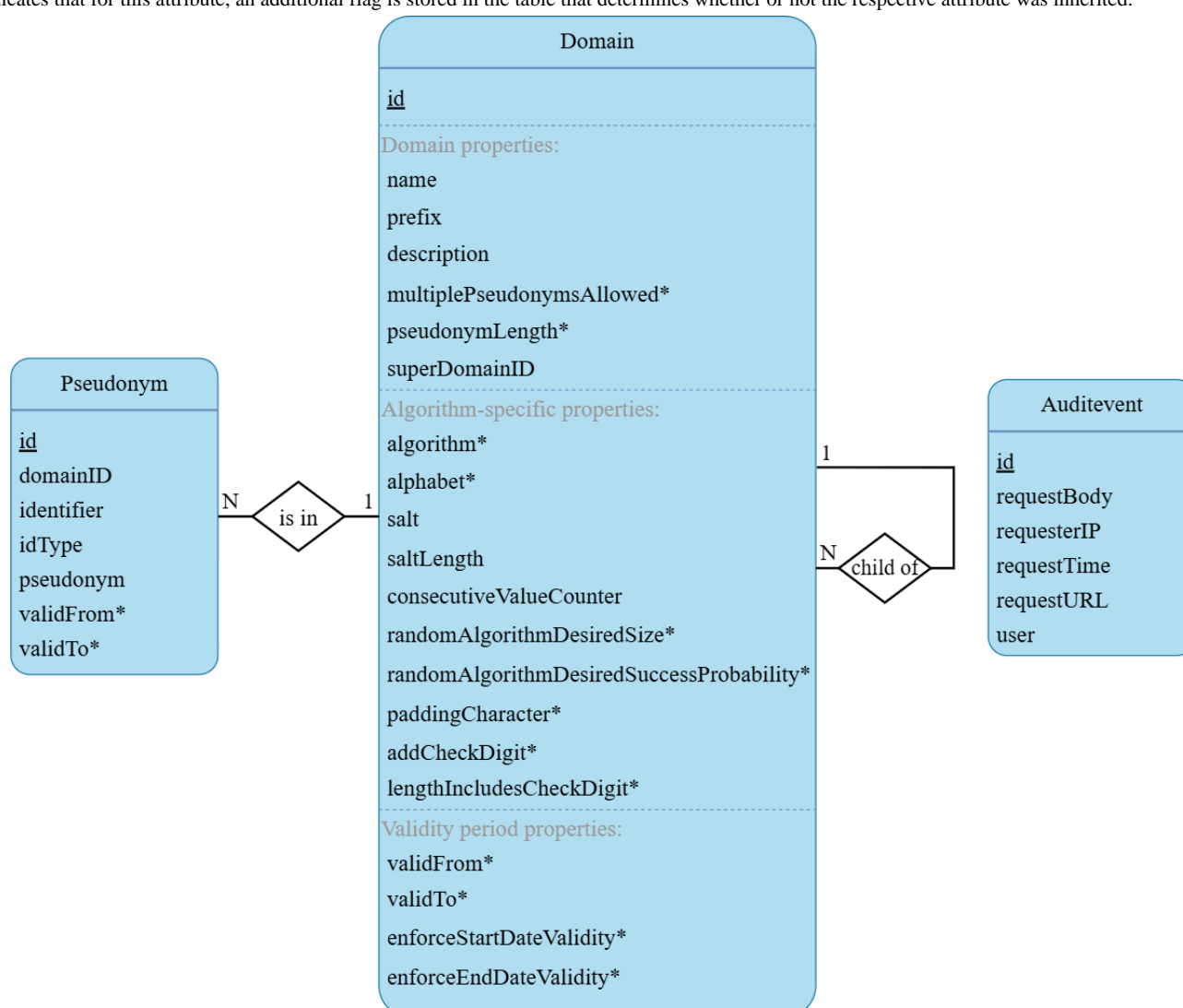
Figure 3. Entity-relationship diagram of the core database design of the Advanced Confidentiality Engine. An asterisk (*) next to an attribute’s name indicates that for this attribute, an additional flag is stored in the table that determines whether or not the respective attribute was inherited.
