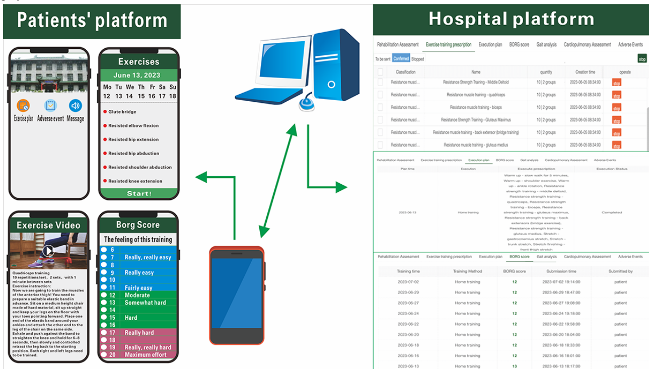
Figure 2. The 3 different parts of the telerehabilitation system (the language of the interface is translated from Chinese). The doctor’s portal can be used to create and modify exercises, monitor training progress, and view patient data. Patients can use the user portal to complete the prescribed exercises and provide feedback to physical therapists. Finally, the transmitter portal encrypts and transmits the data collected, ensuring the overall system’s integrity.
