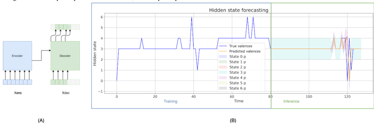
Figure 4. (A) Simplified encoder-decoder architecture of the transformer model. (B) Example of model training and inference. During training, the model learns the parameters to forecast the future state, using the real data as a reference. During inference, the transformer's decoder is responsible for forecasting the future state value in an autoregressive manner. The blue line shows the true states, and the orange line shows those predicted by the model. During inference, the possible future states have associated probabilities, which are illustrated in the graph with different-colored margins around the orange line. Xenc: input sequence for the encoder; Xdec: input sequence for the decoder.
