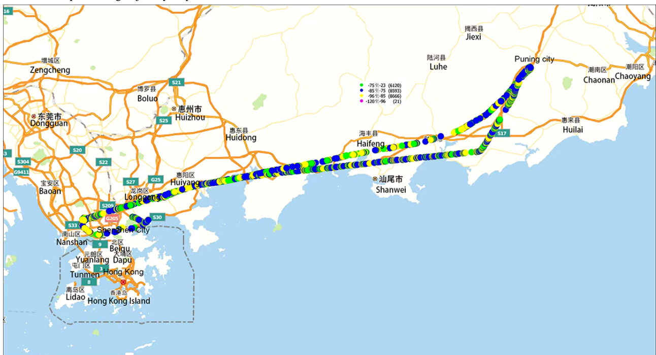
Figure 3. Beidou positioning trajectory map obtained from 5G module.
