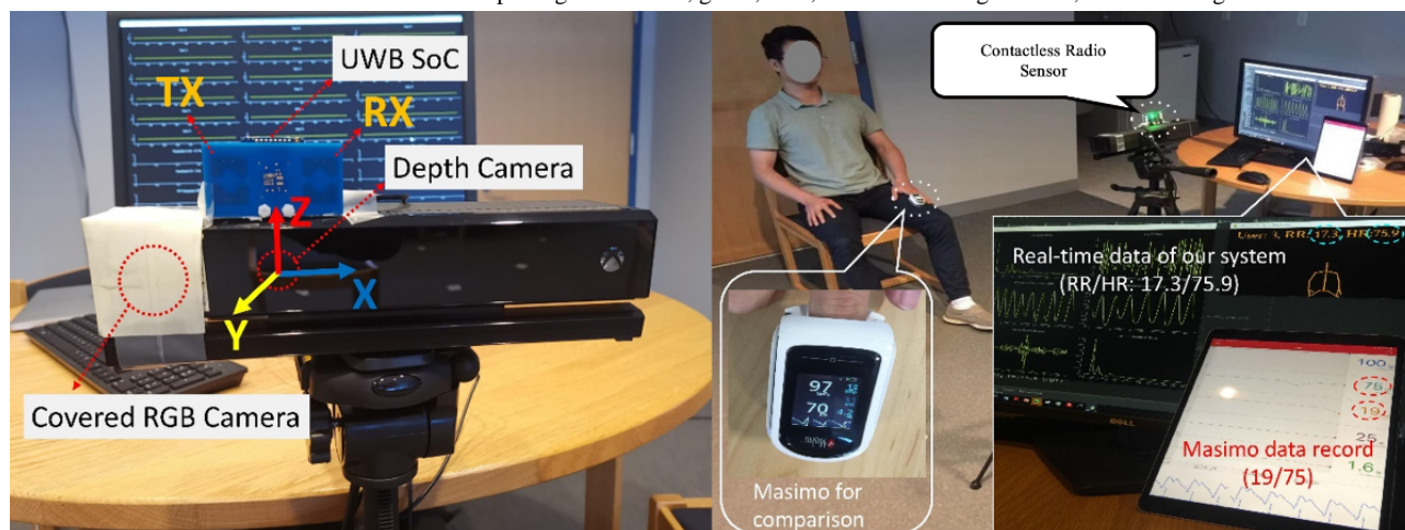
Figure 1. Illustration of a contactless sensor using an ultra-wideband (UWB) radio system on chip (SoC) and a depth camera. The radio waves reflect off the chest and become modulated by respiration and heartbeat movement and are received and processed in order to extract heart rate (HR) and respiration rate (RR). Such contactless sensors can produce results similar to fingertip oximeter pulse readings. This sensor is a prototype that we envision will be housed in a small-form customized hardware package. RGB: red, green, blue; TX: transmitting antenna; RX: receiving antenna.
