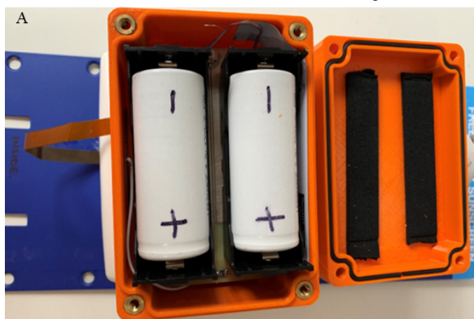
Figure 3. Smart sunscreen station electronic components; the battery housing was protected from water and dust using rubber seals (A), and the BG96 module was connected to a narrowband Internet of Things subscriber identification module (SIM) card and located underneath the battery platform with one NB1 radio antenna attached to the wall of the housing (B).
