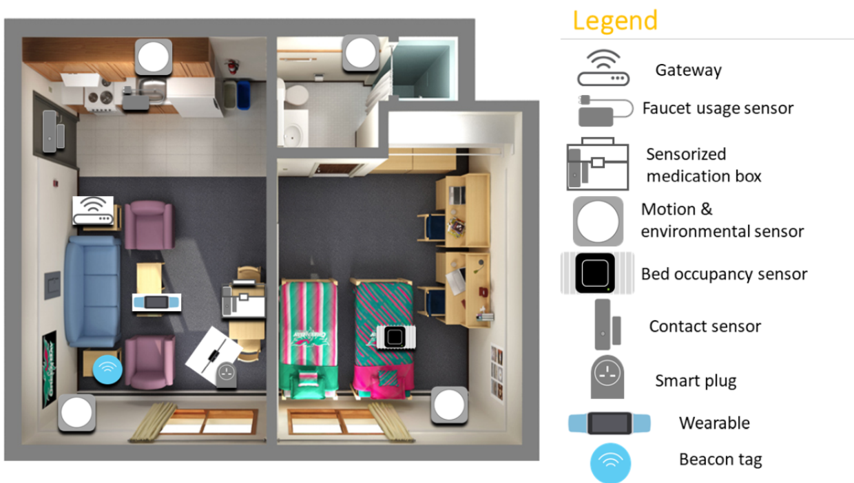
Figure 1. Multimodal sensor set up in homes.
