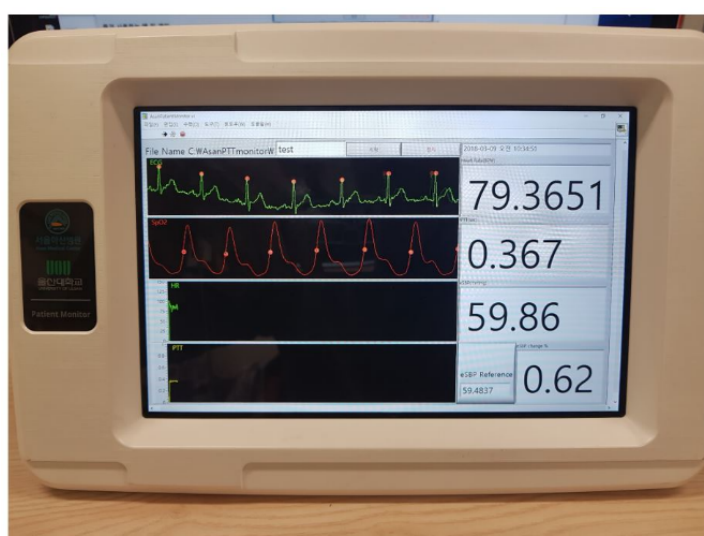
Figure 5. Development of a built-in device to monitor blood pressure surge using electrocardiogram (ECG) and photoplethysmographic (PPG) signal. Tablet personal computer as display and other biosignal sensor system were combined together and enclosed by housing. Blood pressure estimation algorithm was applied to the device, and the software was based on LabVIEW programming. Note that real-time-plotted red dots over ECG and PPG wave on display monitor indicate peak and first derivatives of those signals.
