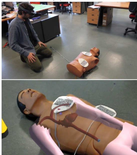
Figure 1. A trainee using the HoloLens device (above) and AR displayed in the trainee's field of view (below).
