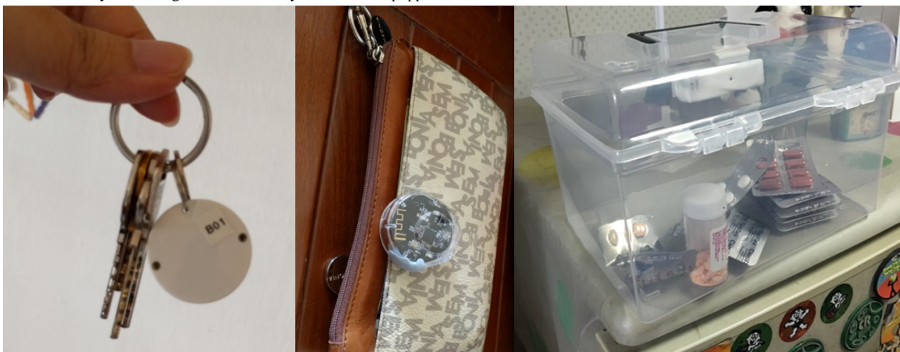
Figure 2. Proximity beacon tags to wallet and keys and sensor-equipped medication box.
