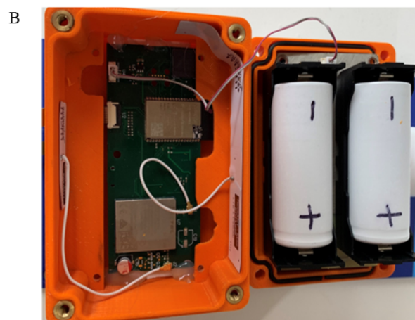
Figure 3. Smart sunscreen station electronic components; the battery housing was protected from water and dust using rubber seals (A), and the BG96 module was connected to a narrowband Internet of Things subscriber identification module (SIM) card and located underneath the battery platform with one NB1 radio antenna attached to the wall of the housing (B).
