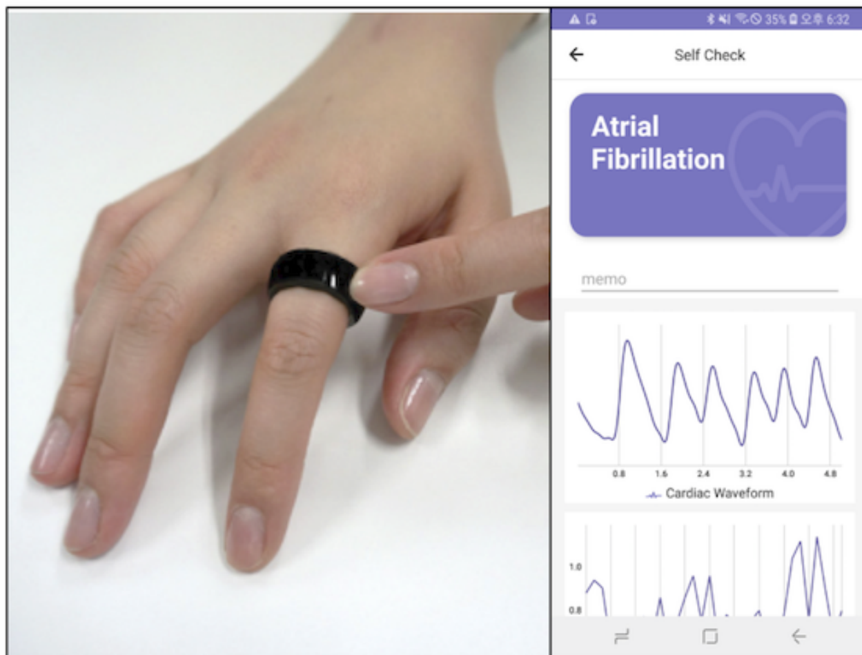
Figure 1. Demonstration of photoplethysmography (PPG) monitoring by CardioTracker (CART). CART measures PPG signals at the proximal phalanx and wirelessly transmits the data to the linked smartphone, which can monitor the PPG signals in real-time, and the deep learning algorithm suggests a possible diagnosis.
