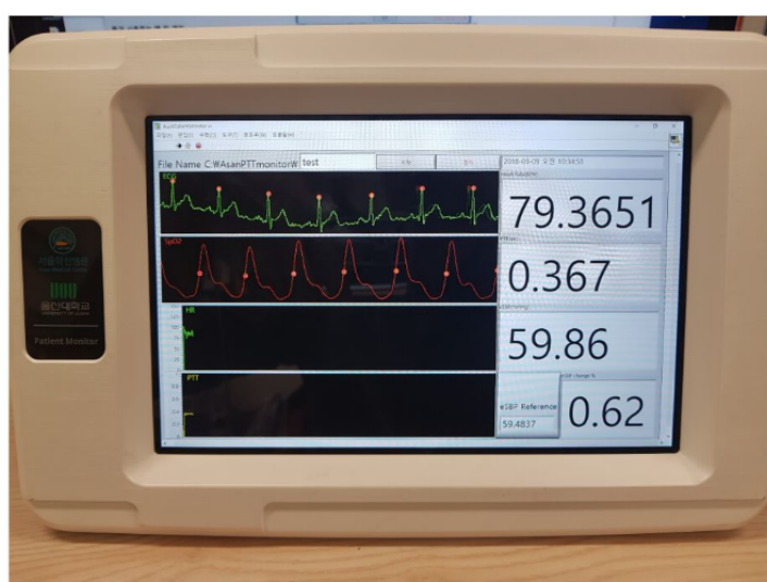
Figure 5. Development of a built-in device to monitor blood pressure surge using electrocardiogram (ECG) and photoplethysmographic (PPG) signal. Tablet personal computer as display and other biosignal sensor system were combined together and enclosed by housing. Blood pressure estimation algorithm was applied to the device, and the software was based on LabVIEW programming. Note that real-time-plotted red dots over ECG and PPG wave on display monitor indicate peak and first derivatives of those signals.
