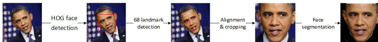
Figure 1. Pre-processing workflow to obtain chip images to use as inputs in the convolutional neural network, showing the intermediate results. Image courtesy Barack Obama Presidential Library [22].
