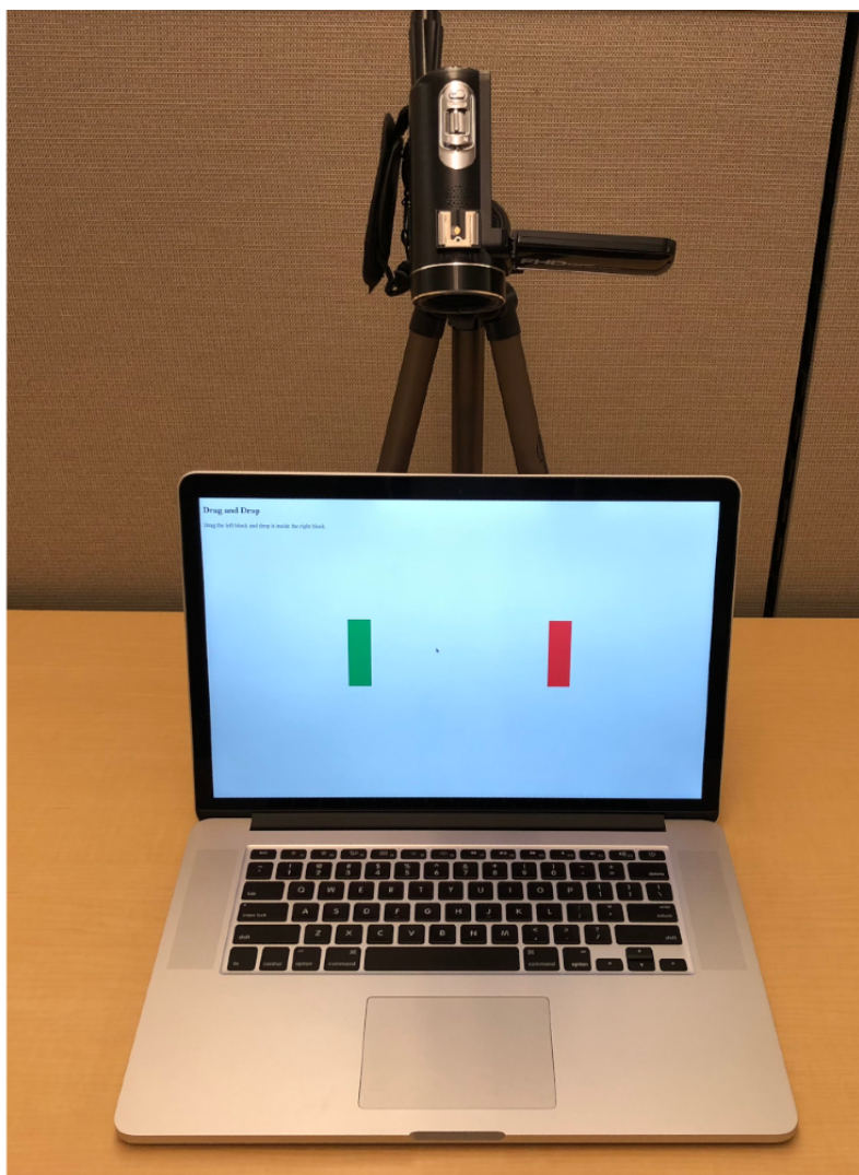
Figure 3. Apparatus: a 15-inch 2015 MacBook Pro (Apple Inc) with a passive movement logger teamed with an overhead camera for the ancillary recording of hand movement.
