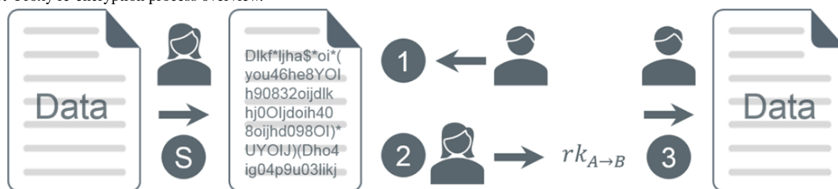
Figure 3. Proxy re-encryption process overview.
