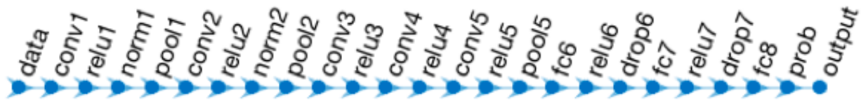
Figure 1. The architecture of AlexNet, which comprised 25 layers.
