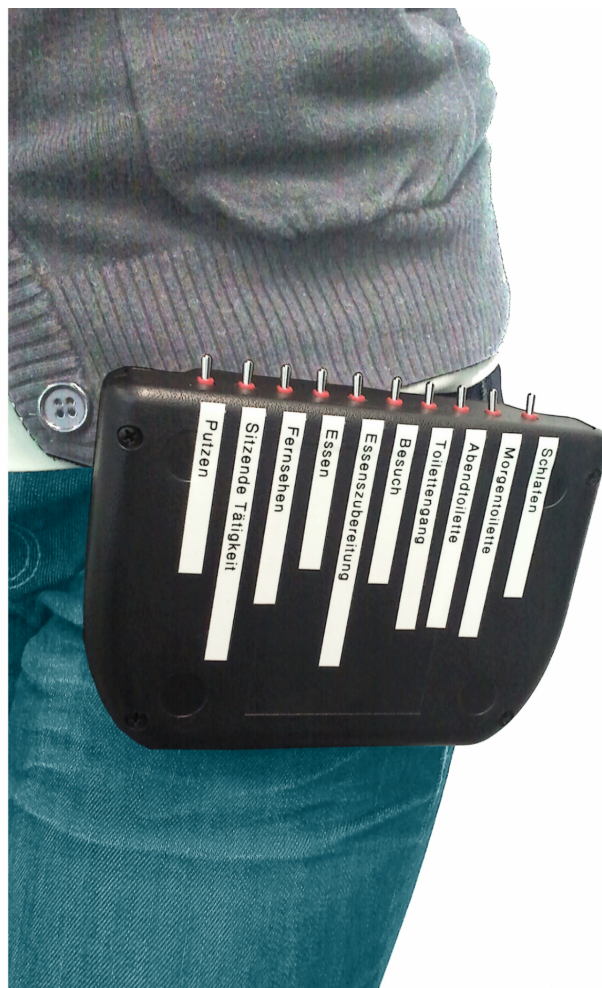
Figure 3. Wireless protocol device worn by participant (switches on top of the box are labeled with 8 different activities such as “watching TV” or “sleeping”).
