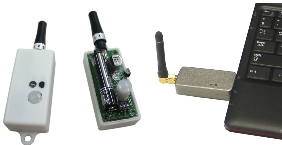
Figure 1. Wireless sensor box with housing (left) and an inside view of the same sensor box (middle) displaying PCB board with environmental sensors and primary cell; receiver unit with antenna (right) is connected to the central computer unit serving as a data server and Web link (between the two devices a bidirectional data transmission is established).
