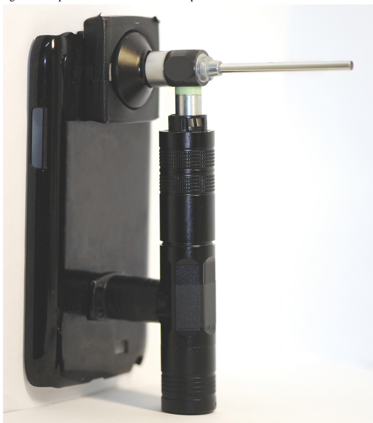
Figure 3. Prototype of a self-designed smartphone-based otorhinoendoscope.
