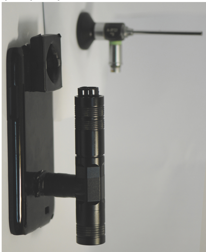
Figure 2. Self-designed specific adapter with portable light source.
