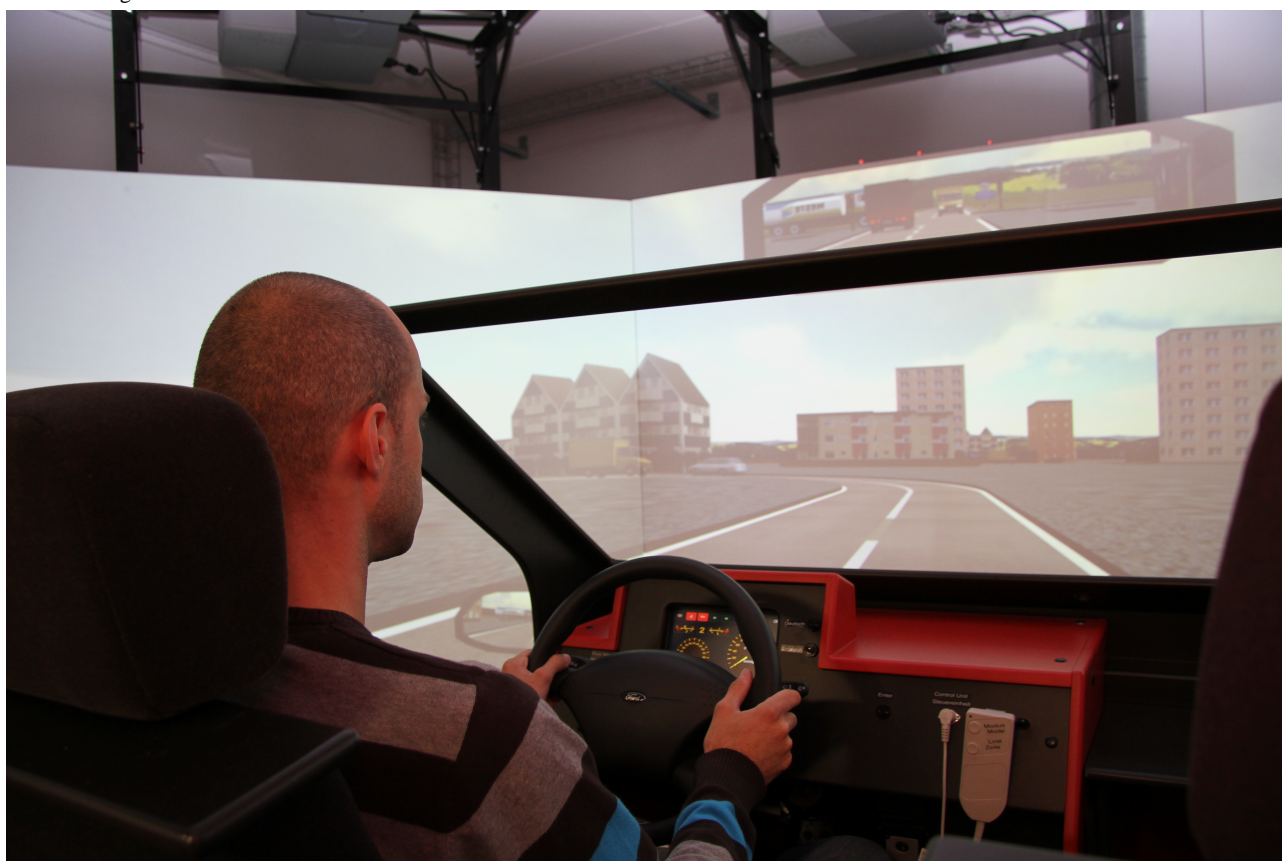
Figure 2. High-fidelity fixed-frame driving simulator with younger test subject. The steering wheel, cockpit, and parts of two projection screens with the virtual driving screen are shown.
